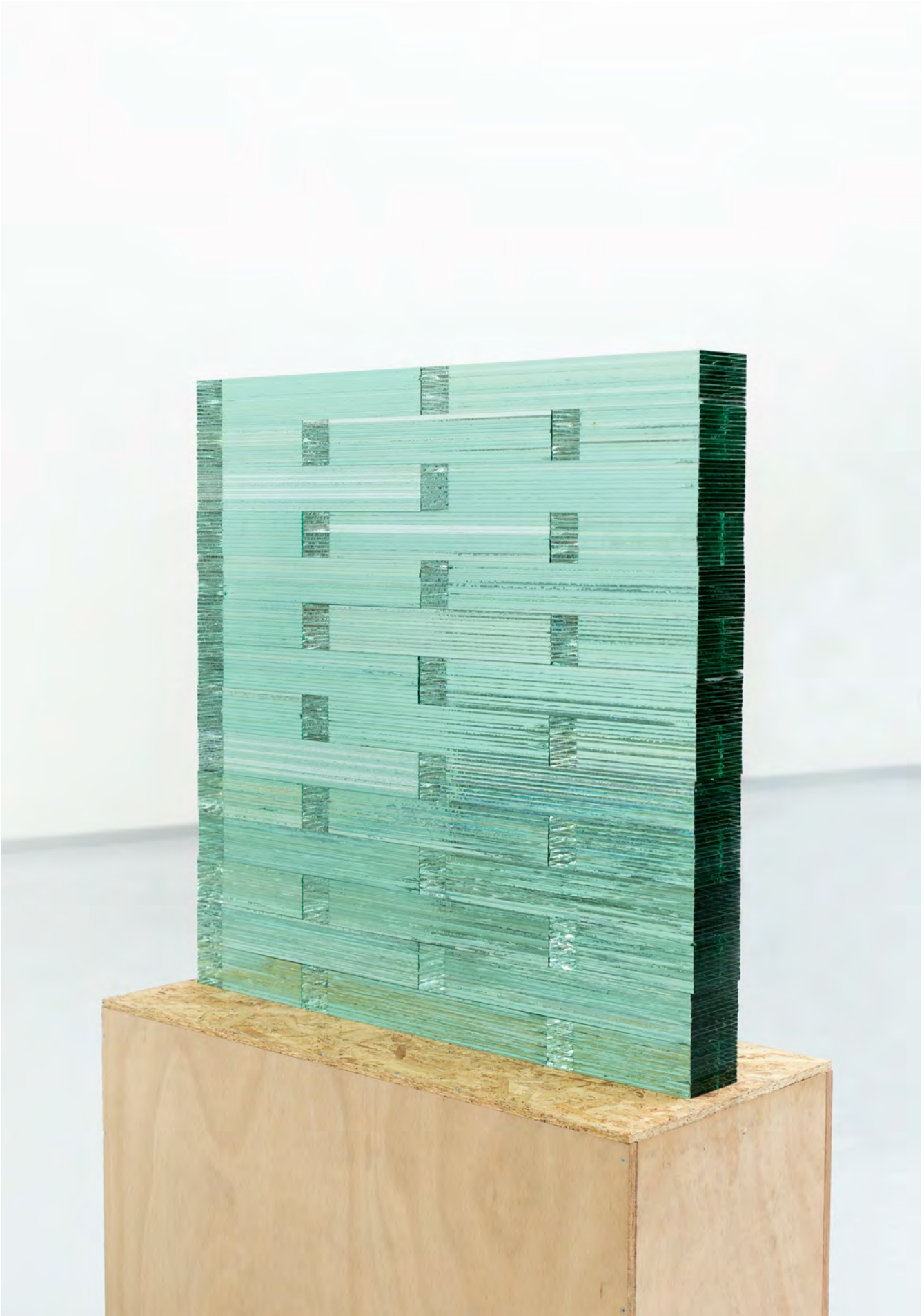
Figure 24/ Prototype built from glass bricks
