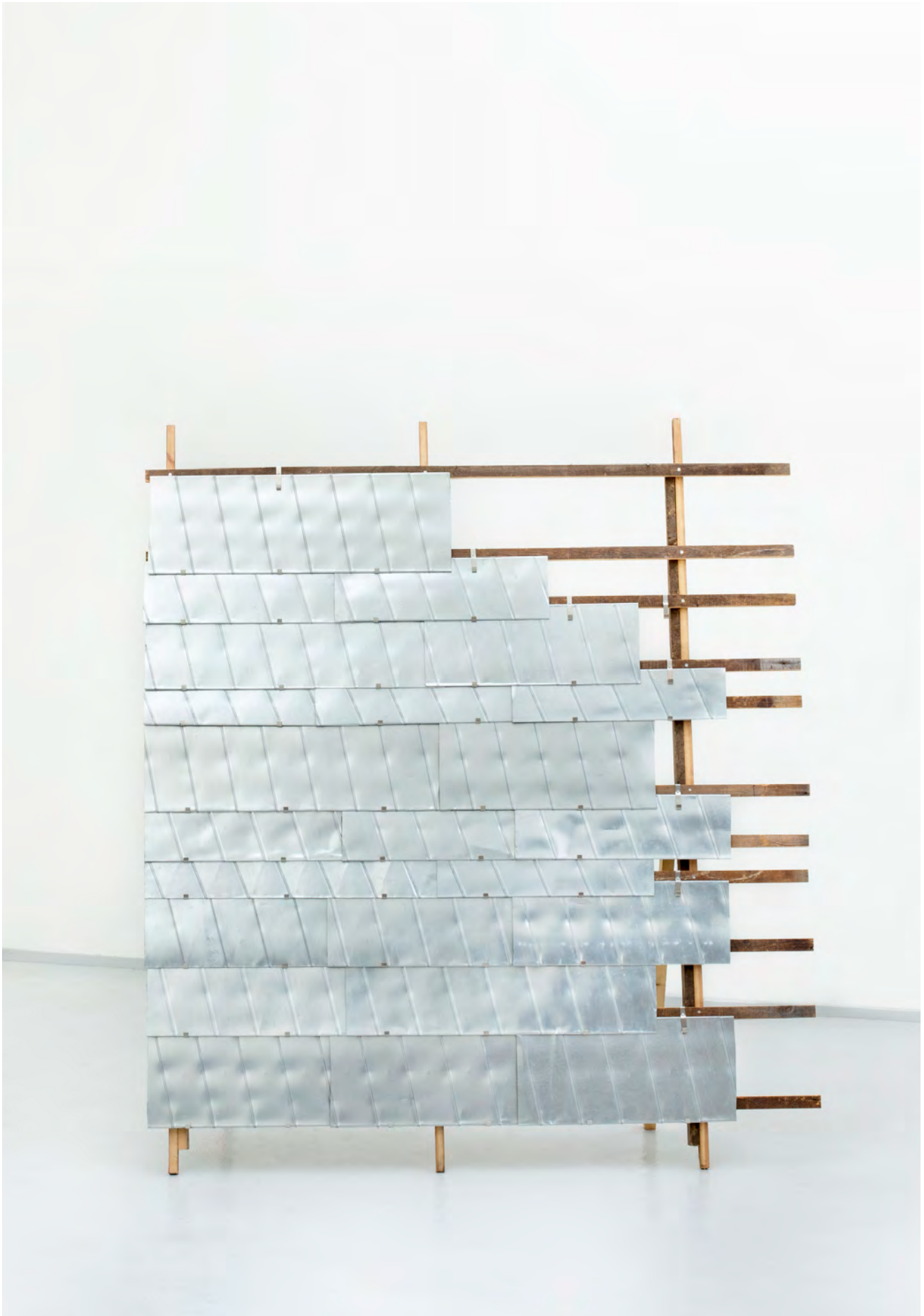
Figure 31/Prototype of Spiro Wall made from flattened ventilation ducts
