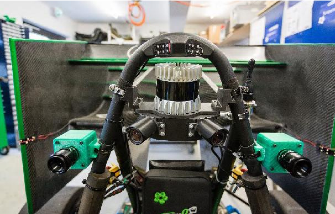
The 3D stereo vision deployed on the autonomous race cars. Image credit: Nerian.
