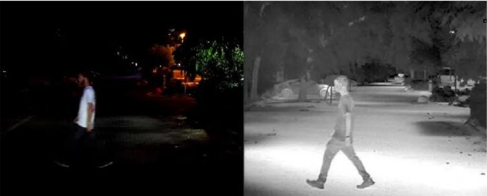
A pedestrian crossing a dark suburban street. Visible light camera vs. FLIR® thermal camera captured by Foresight’s test vehicle. Image credit: Foresight.
