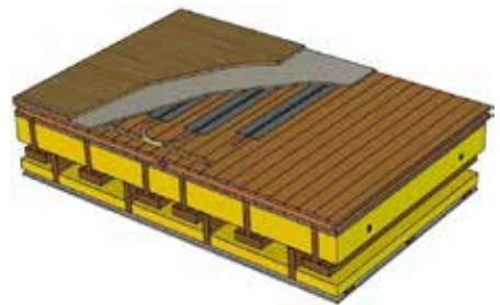
Horizontal panel showing hydronic heating channels.
