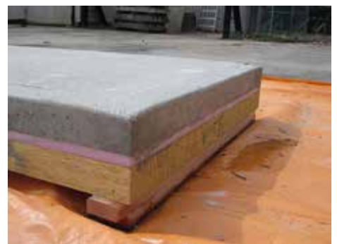
Composite floor panel used for testing. Photo Credit: Equilibrium Consulting Inc.
