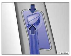
Fig. 59 Next to the front seats: Safety belt height adjuster.
