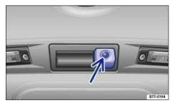
Fig. 151 In the rear hatch: Location of the Rear Assist camera.
