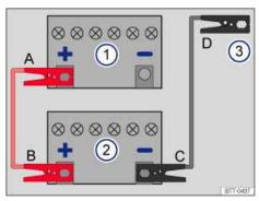
Fig. 200 Diagram for attaching the jumper cables: Dead battery 1 and booster battery 2.
