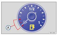
Fig. 157 In the instrument cluster: Fuel gauge.
