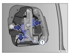
Fig. 199 In the side of luggage compartment: Removing the bulb holder.
