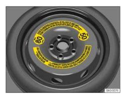
Fig. 112 In the luggage compartment: Compact spare wheel.
