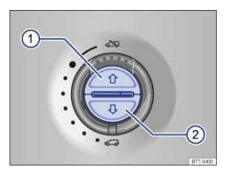
Fig. 35 In the headliner: Buttons for the sunshade
