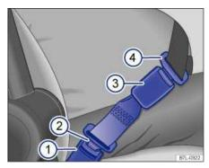
Fig. 60 A safety belt extender properly attached to the factory-installed safety belt.
