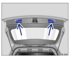
Fig. 32 Opened rear hatch: Recessed grips for closing.
