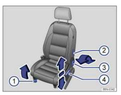
**Fig. 38** Driver seat: Manual controls to move the seat forward or back and adjust the backrest angle, seat height, and lumbar support (if applicable).
