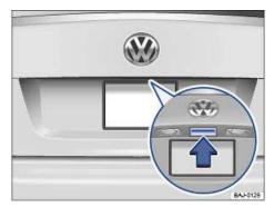
Fig. 31 Opening rear hatch from the outside.
