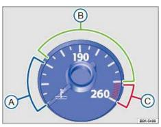
Fig. 165 Engine coolant temperature gauge in the instrument cluster: A Engine cold; B Normal temperature range: C Warning zone.
