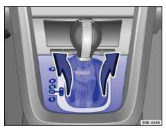
Fig. 179 Removing the selector gate cover.
