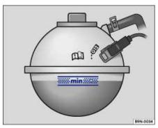
Fig. 166 Coolant expansion tank in the engine compartment.
