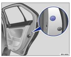
Fig. 176 On the front side of the right rear door: Emergency lock, covered by a rubber seal.
