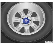
Fig. 111 In the luggage compartment: Handwheel holding the spare wheel in place.
