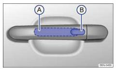
Fig. 27 Keyless Access locking and starting system: Sensor for unlocking A on the inside of the front door handles. Sensor for locking B on the outside of the front door handles.
