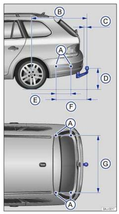
Fig. 107 Dimensions and attachment points for retrofitting a trailer hitch.
