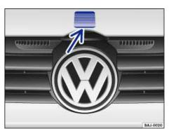
Fig. 162 Above the radiator grille: Outside engine hood release.
