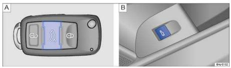
Fig. 30 A: Button in the remote control vehicle key to unlock the rear hatch. B: Button in the driver door to unlock the rear hatch.
