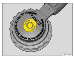
Fig. 145 In the engine compartment: Brake fluid reservoir cap.
