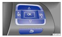
Fig. 16 Right side of the multi-function steering wheel (if equipped): Controls for the menus in the instrument cluster.
