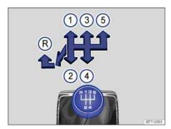
Fig. 138 Gearshift pattern of a 5-speed manual transmission.
