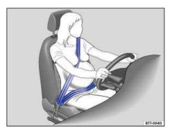
Fig. 58 Proper safety belt positioning for expectant mothers.
