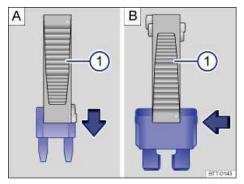
Fig. 195 Removing or inserting a fuse using the plastic tweezers 1.
