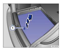
Fig. 181 In the luggage compartment: Lifting up the floor panel.
