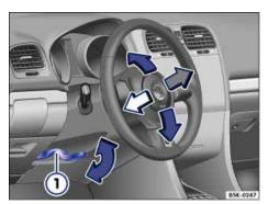
Fig. 44 Manual adjustment for the steering wheel position.
