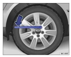
Fig. 188 Changing a wheel: Loosening wheel bolts.
