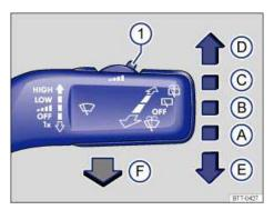
Fig. 89 Operating the front windshield wipers.
