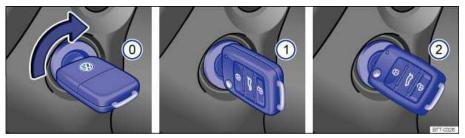
Fig. 132 In the ignition switch: Vehicle key positions.
