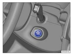
Fig. 133 On the right side of the steering column: Starter button for the Keyless Access locking and starting system.
