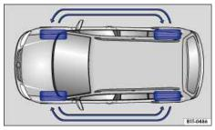
Fig. 108 Tire rotation diagram.
