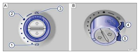
Fig. 34 In the headliner: Rotary switch for the power sunroof. A: Turn the rotary switch to slide the sunroof open or closed. B: Press or pull the switch to tilt open or to close.
