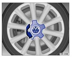
Fig. 185 Twisting the hubcap off.
