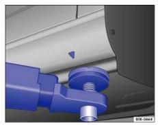
Fig. 172 Front lift point for workshop hoist or floor jack.
