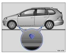
Fig. 189 Lift points for the jack.
