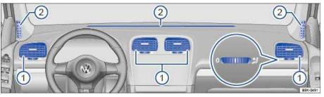
Fig. 156 In the instrument panel: Air vents
