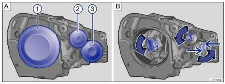
Fig. 196 In the engine compartment: Covers in the left headlight assembly. 1 Low beam, 2 Turn signal indicator, 3 High beam and parking light as well as daytime running light.
