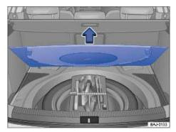
Fig. 182 In the luggage compartment: Spare wheel and vehicle tool kit
