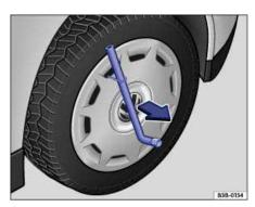
Fig. 187 Pulling the wheel cover off.
