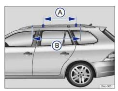
Fig. 105 Roof fails: Base carrier attachment areas.
