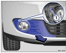
Fig. 197 In front right bumper: Removing the light assembly.
