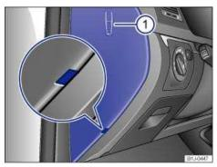
Fig. 192 On the driver side in the instrument panel: Fuse box cover with plastic tweezers 1 on the inside of the cover.
