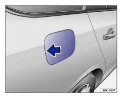
Fig. 158 Right rear side of vehicle: Opening the fuel filler flap.
