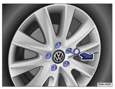
Fig. 186 Pulling cover caps off wheel bolts.
