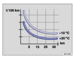
Fig. 147 Fuel consumption in I/100 km at 2 different outside air temperatures.
