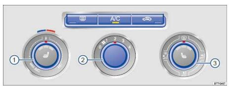
Fig. 154 In the center console: Manual A/C controls.
