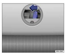
Fig. 178 Inside the luggage compartment: Opening the rear hatch.
