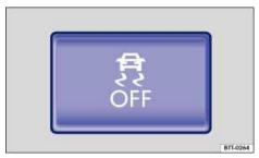
Fig. 144 In the center console: Button for switching ASR on and off manually.
