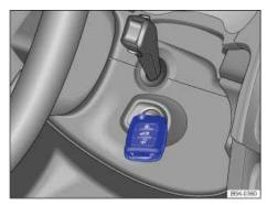
Fig. 134 Hold the remote control vehicle key to the right of the steering column: Emergency starting feature on vehicles with Keyless Access.
