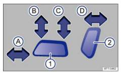
Fig. 39 Driver seat: Electrical controls to move the seat backward or forward, and adjust seat cushion height and backrest angle (if applicable).
