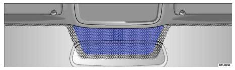
Fig. 88 Heat-reflective windshield with communications window (blue shaded area).
