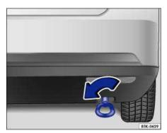
Fig. 203 In the rear right bumper: Screwing in the towing lug.
