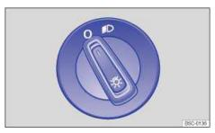
Fig. 84 Headlight switch next to the steering wheel.
