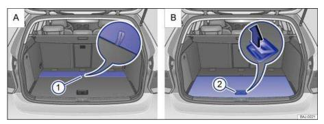
Fig. 103 In the luggage compartment: Opening the luggage compartment floor.
