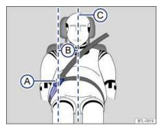
Fig. 61 Positioning of the safety belt extender.
