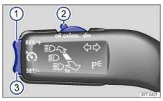
Fig. 150 On the left side of the steering column: Cruise control buttons and switches.
