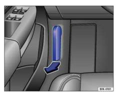
Fig. 161 In the footwell on the driver side: Inside engine hood release lever.
