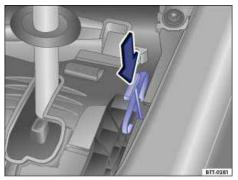
Fig. 180 Releasing the selector lever lock.
