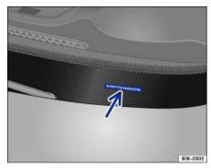
Fig. 18 Vehicle identification number (VIN).
