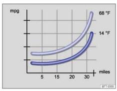
Fig. 146 Fuel consumption in mpg at 2 different outside air temperatures.
