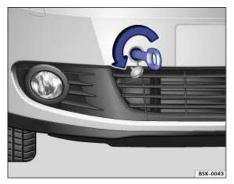
Fig. 202 In the right front bumper: Screwing in the towing eye.
