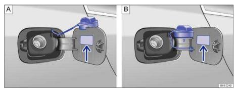
Fig. 159 Fuel cap placed on the open fuel filler flap: Versions A and B.
