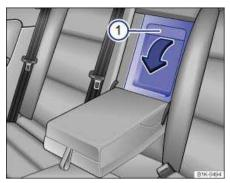
Fig. 99 In the rear seat backrest: Opening the luggage compartment pass-through.
