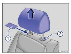
Fig. 42 Removing the front head restraints.
