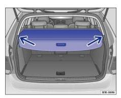
Fig. 97 In the luggage compartment: Closing the luggage compartment cover.
