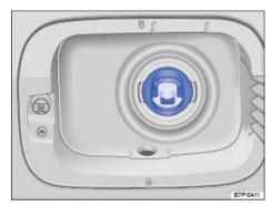
Fig. 160 With open fuel cap: Misfueling guard in the fuel filler neck.
