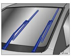
Fig. 91 Windshield wiper in service position.
