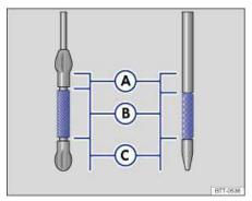
Fig. 163 Oil dipstick with engine oil level marks.
