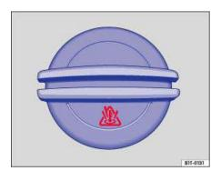
Fig. 167 Coolant expansion tank cap in the engine compartment.
