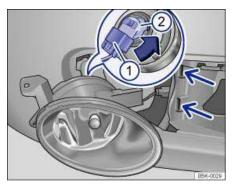
Fig. 198 Replacing a light bulb in the fog light.
