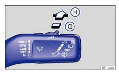
Fig. 90 Operating the rear wiper.
