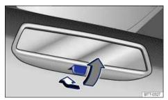
Fig. 93 Manually adjustable inside mirror.
