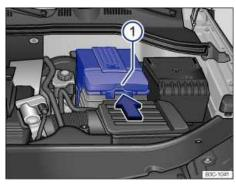
Fig. 168 In the engine compartment: Remove the cover from the vehicle battery.
