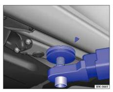
Fig. 173 Rear lift point for workshop hoist or floor jack.
