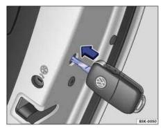
Fig. 177 On the front side of the right rear door: Locking the vehicle with the key bit in the vehicle key.
