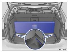
Fig. 104 In the luggage compartment: Upright position of the luggage compartment floor.
