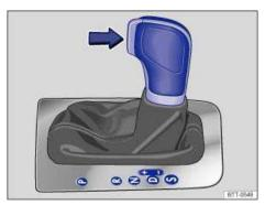
Fig. 140 Side view: Automatic transmission selector lever with shift lever release button (arrow).
