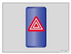
Fig. 174 In the center of the instrument panel: Button for the emergency flashers.
