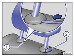
Fig. 43 Removing the rear head restraints.
