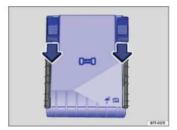
Fig. 193 In the engine compartment: Fuse box cover.
