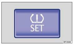
Fig. 114 In the glove compartment: SET button for the Tire Pressure Monitoring System.
