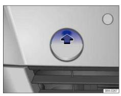
Fig. 201 In the right front bumper: Removing the cover.
