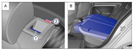
Fig. 96 A Rear seat bench: release button 1, red mark 2. B Seat backrest folded forward.
