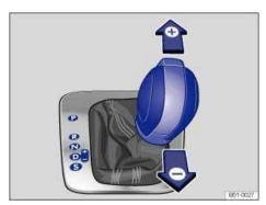
Fig. 142 Selector lever in Tiptronic position.
