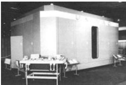
Figure 1-14 - UNIVAC I, the first commercial electronic computer, achieved 1900 operations per second in a smaller and more efficient package than ENIAC
