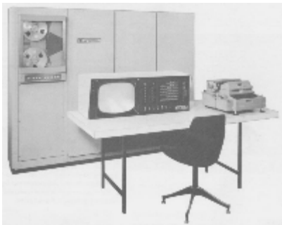
Figure 1-17 - Digital Equipment Corporation's first computer was the PDP-1. It was built mostly of DEC 1000-series system modules, using Micro-Alloy and Micro-Alloy-Diffused Transistors
