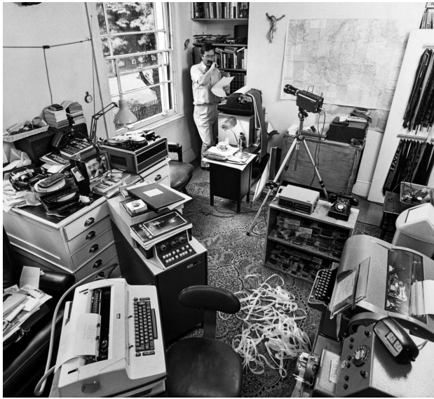
2. Len Deighton at work on Bomber in his high-tech home office at 29 Merrick Square, London, in 1968. The MT/ST is visible in the foreground. Also visible are his Selectric typewriter with its roll of telex paper atop the improvised standing desk, residue from the telex paper littering the floor (and the telex machine itself to the right), and a map of North Central Europe (the setting for the book) on the far wall.
