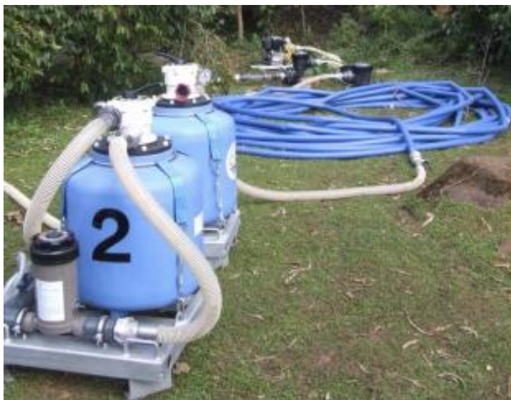
Skid mounted water treatment unit, in Ethiopia, showing pump in background with suction side coagulant dosing, flexible pipe for flocculation, pressurized sand filters in foreground and chlorine doser at front, (IFRC LMS Unit – capacity 4,000 liters/hour)
