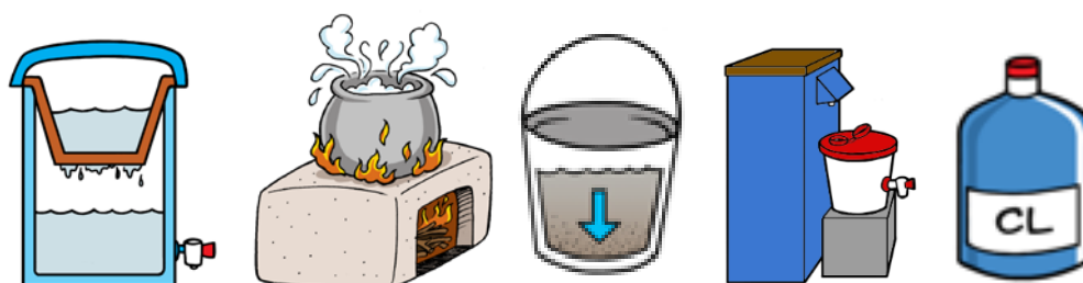
Examples of HWTS options: ceramic pot, boiling, settling, biosand filter, and liquid chlorine.
