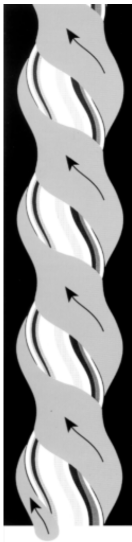
Figure 2.1 Progressive cavity pumping method
