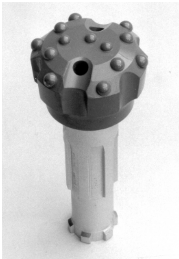
Figure 1.2 Down-the-hole-hammer tungsten button drill bit
