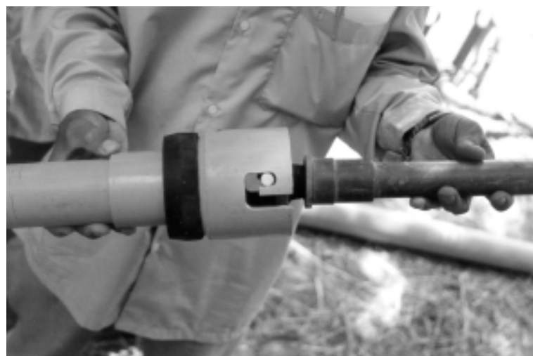
Figure 6.10 Placement of telescopic screen using simple bayonet tool
