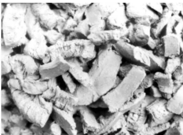
Figure 2.9 Individual clay cuttings washed to the surface
