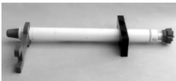
Figure 3.3 Down-the-hole hammer – with stripping clamp and spanner
