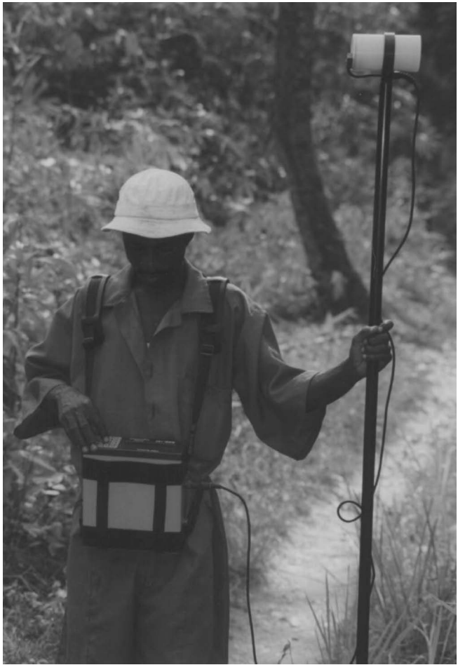
Figure 5.27 The proton precessor magnetometer in use in Nigeria. Photo: BGS, © NERC 2000.
