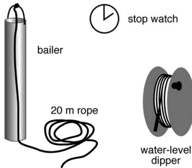
Figure 7.7 Equipment required to carry out a bailer test.
