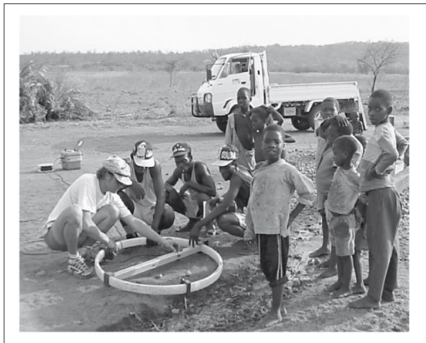
Figure 5.57: Setting up a TDEM measurement (Mozambique, 2000).
