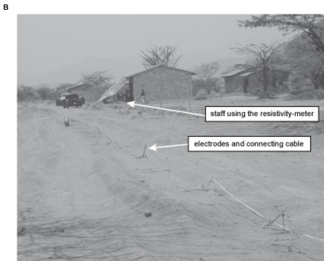
Figure 5.30: ERI measurement array.
